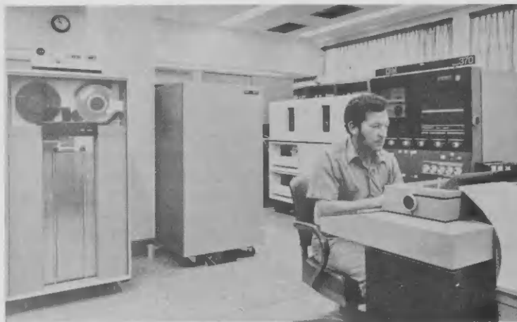
Senior Computer Operator Pedro Yarzagaray of MCS-Data Processing Group, is shown here at the new IBM 370 Console. At left is one of the four automatic magnetic tape drives, model 3420. At right is the Computer Processing Unit.
